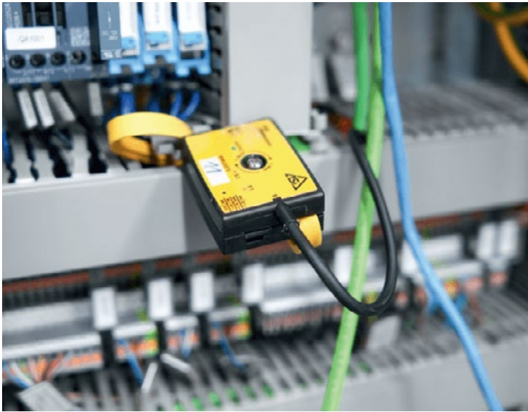
Active Distributor Asi Safety BWU3373 from Bihl+Wiedemann for integrating safety switches into the ASi network.
